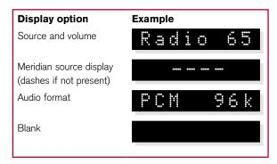
The audio format display shows PCM, Data, or MHR followed by the frequency, or NL (not locked).
