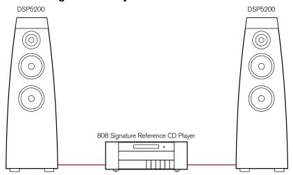
Meridian DSP loudspeakers include DSP volume and tone controls, and be connected directly to digital sources, such as the 808 Signature Reference CD Player, to create an compact high-quality music system.
