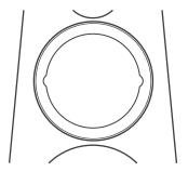
Hold the ring by one of the indentations by depressing the grille fabric with your thumb, and then wiggle the ring forwards until it comes free of the speaker. The grille fabric is very resilient and any depressions will soon disappear.
