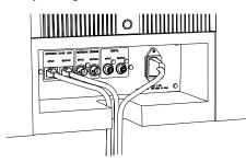
Finally refit the cover plate into position, concealing the input/output panel and connections.
