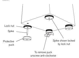
On carpeted floors all parts can be fitted and the spike should be adjusted so that it extends through the puck and penetrates the carpet pile to the floor underneath. Where a carpet has a deep pile you can fully unscrew and remove the puck to expose more of the spike. Once the speakers are upright in their playing positions adjust the spikes until the loudspeakers are stable and tighten the lock nuts to prevent the spikes moving in the cabinet.
