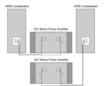
Extremely high sound quality can be achieved using two separate 557 Power Amplifiers, one to drive each loudspeaker. The two channels in each amplifier are used to drive the LF and HF units in each loudspeaker.
