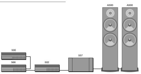
The digital output provided by the 500 Compact Disc Transport can be decoded by the 566 20-bit Digital to Analogue converter to provide a high-quality audio output for use with a conventional audio preamplifier. The 566 20-bit Digital to Analogue Converter can also decode digital signals from other sources, including LaserDisc players and Digital Audio Tape.
