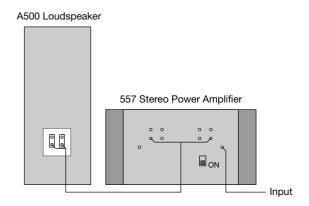
You can use the 557 as a mono power amplifier, to obtain more than three times the power output, by wiring it in bridge mode.
