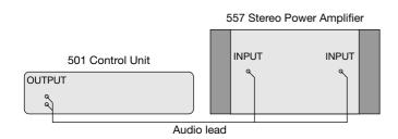
Connect the sockets marked OUTPUT L and R on the back panel of the 501 Control Unit to the INPUT sockets on the back panel of the 557 Stereo Power Amplifier.
