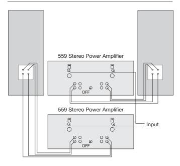
Extremely high sound quality can be achieved using two separate 559 Stereo Power Amplifiers, one to drive each loudspeaker. The two channels in each 559 Stereo Power Amplifier are used to drive the LF and HF units in each loudspeaker.
