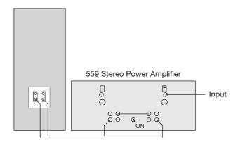
You can use the 559 as a mono power amplifier, to obtain more than three times the power output, by wiring it in bridge mode.
