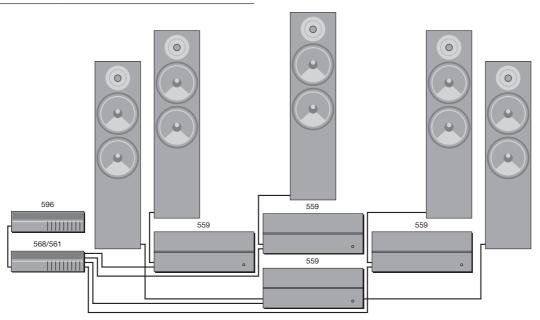
559 Stereo Power Amplifiers are ideal for use with the Meridian 561 Digital Surround Controller or the 568 Digital Surround Processor, to drive five passive loudspeakers in a high-quality surround system. The recommended configuration, shown above, uses three 559 Stereo Power Amplifiers operating in
