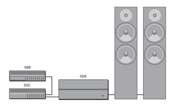
The 588 Compact Disc Player is ideally suited for use with the Meridian 559 Stereo Power Amplifier and passive loudspeakers, with control over the volume and source selection provided by the 502 Analogue Controller. These units provide balanced inputs and outputs, allowing a completely balanced system to be created.
