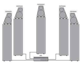
The ultimate Meridian Digital Theatre uses a 565 in conjunction with four or six DSP6000 Digital Loudspeakers and a DSP6000C Digital Centre Loudspeaker.
