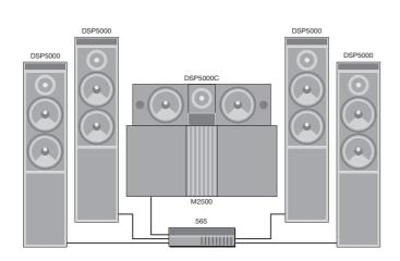
The Meridian Digital Theatre is a completely digital system which provides audiophile-quality surround sound for music and film. Two pairs of DSP5000 Digital Loudspeakers are complemented by a DSP5000C Digital Centre Loudspeaker and an M2500 Active Subwoofer.
