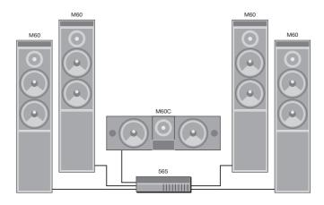
The ultimate analogue surround system consists of two pairs of Meridian M60 Active Loudspeakers, in conjunction with a Meridian M60C Active Loudspeaker. These speakers can be connected directly to the 565 to provide a complete five-speaker surround system.
