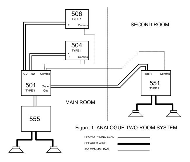
To set up the 551 in the second room, simply follow the TYPE procedure outlined in the *User Manual* and set it to TYPE 7. Because the second room is connected to the tape output of the 501, the second room source can be changed with the **COPY** key on the 501. Alternatively, a 551 in both rooms or a 501/555 combination in both rooms may be used. The control unit in the second room is set to TYPE 7.
