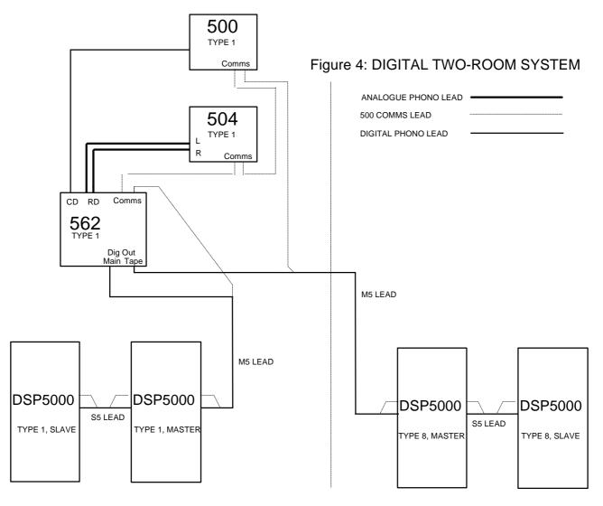
The 562 contains one analogue to digital converter, so only one analogue source may be listened to at any one time. Otherwise the functionality is the same as any other Two-Room system.
