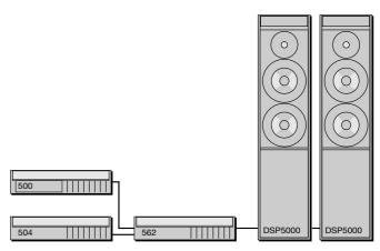
The 500 Compact Disc Transport provides a precision digital output, and can drive DSP5000 Digital Loudspeakers directly.
