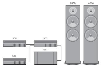
The 508 20-Bit CD Player is an integrated CD transport and converter, providing both digital and analogue outputs.
