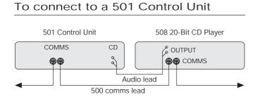
Connect the sockets marked OUTPUT L and R on the back panel of the CD player to the CD input on the back panel of the 501 Control Unit.
