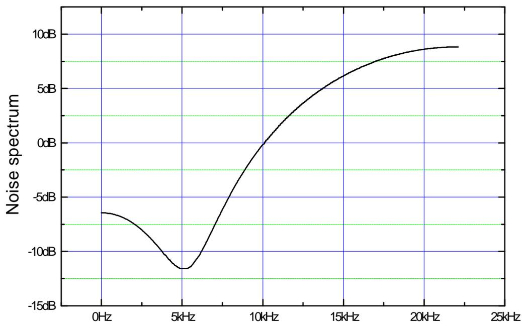
Above: noise spectrum for Shape A at 44.1kHz.
