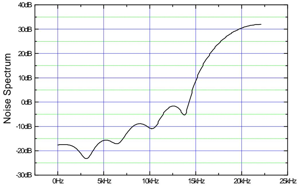
Above: noise spectrum for Shape B at 44.1kHz
