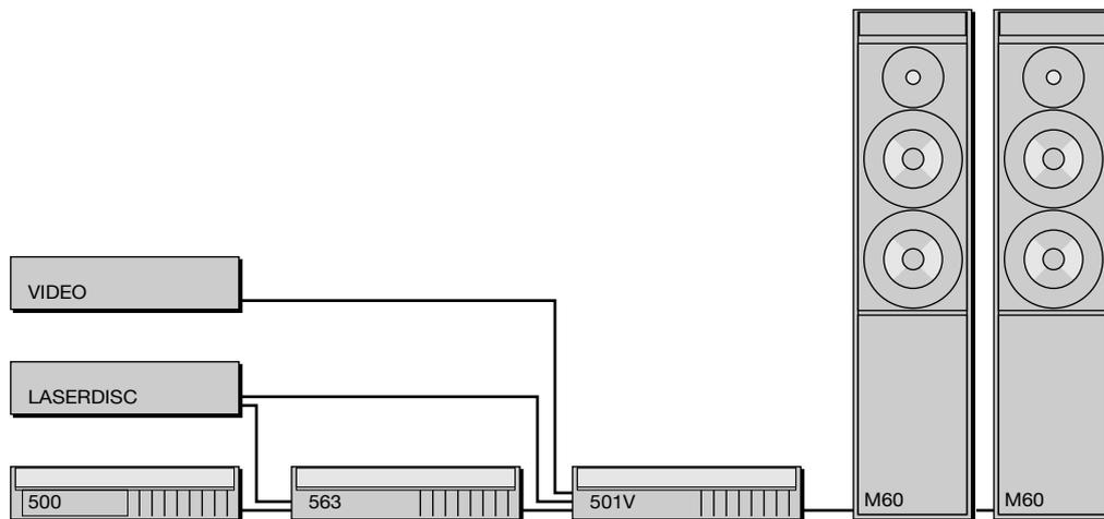
The digital output provided by the 500 Compact Disc Transport can be decoded by the 563 Digital to Analogue converter to provide a high-quality audio output for use with a conventional audio preamplifier.
