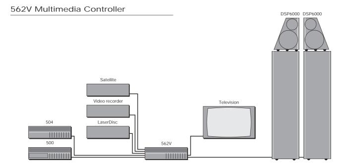
The 562V Multimedia Controller is the ideal control unit for use with the Meridian DSP6000 Digital Loudspeakers.
