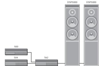
The 500 Compact Disc Transport provides a precision digital output, and can drive Meridian DSP5000 Digital Loudspeakers directly.
