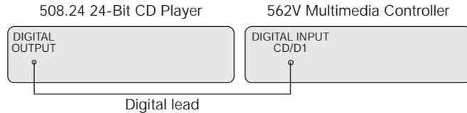
You can connect up to five digital and two optical sources to the 562V Multimedia Controller.
