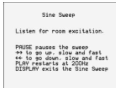
The Sine Sweep test signal allows you to check your room for rattles and buzzes which could interfere with your listening.
