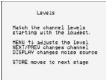
This test allows you to adjust the output level to each speaker individually, and it follows the general guidelines from Dolby and Lucasfilm. A Sound Pressure Level (SPL) meter can be useful at this stage; ask your dealer for more information.
