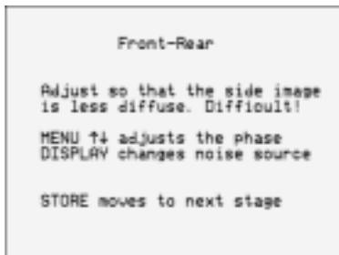
This calibration test adjusts the relative phase between the front speakers and the rear surround speakers.
