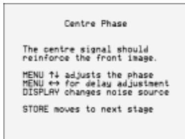
As in the previous test, signals are applied to the main left, right, and centre speakers to allow you to adjust the relative phase and delay on the centre channel.
