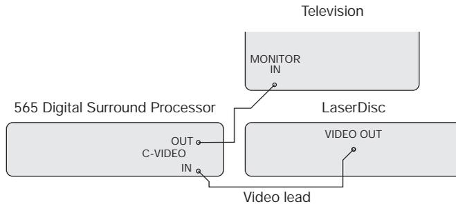
If your surround system includes a television the 565 can add a text overlay to the video signal, to provide additional information about its operation in the form of a textual on-screen display (OSD). In normal operation this repeats the information provided on the 565 front panel display. During calibration the on-screen display provides additional guidelines to help you perform the calibration sequence.
