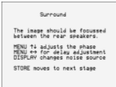
This test presents the Low test signal through the left and right rear surround speakers to allow you to adjust the relative phase and delay between them.
