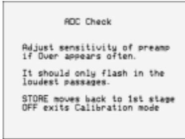
This test provides metering to help you set the level of the analogue inputs. The analogue-to-digital converter (ADC) fitted for the analogue input to the 565 has a sensitivity of 2V rms for full scale. With this setting, the analogue input can be connected to the output of a LaserDisc or CD player and will not require adjustment. If the analogue signal comes from a preamplifier or control unit, then it is important to ensure that the internal ADC is not overloaded.
