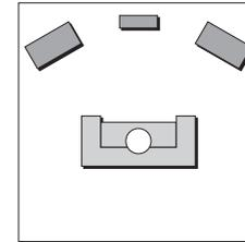
Adding a centre speaker is the most significant step you can take to upgrade a two-speaker system, whether you are using the system for cinema, music, or a combination of the two. It reinforces the central image, and allows the left and right speakers to be further apart for a wider soundstage. This gives a more realistic and stable three-dimensional image of the original recorded sound, for outstanding music and cinema reproduction.
