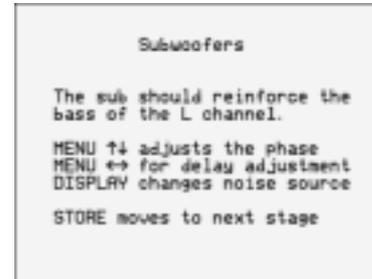
In this calibration test the Low noise signal is used to allow you to calibrate the phase and delay of each subwoofer in turn relative to another reference speaker. The reference chosen depends on the layout.
