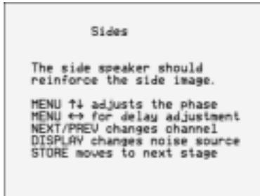
If your layout includes side surround speakers an additional Sides option allows you to adjust the relative phase and delay. Side L presents the signal to the front left, rear left, and side left speakers and you adjust the phase of the side left speaker for reinforcement, as with Centre Phase. Side R repeats the test for the three right speakers.
