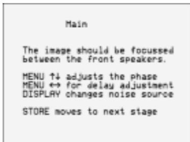
This test allows you to set the relative phase and the relative delay between the left and right main speakers.
