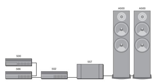
The digital output provided by the 500 Compact Disc Transport can be decoded by the 566 24-Bit Digital to Analogue Converter to provide a high-quality audio output for use with a conventional audio preamplifier. The 566 24-Bit Digital to Analogue Converter can also decode digital signals from other sources, including LaserDisc players and Digital Audio Tape.
