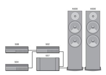
The 508 24-Bit CD Player is an integrated CD transport and converter, providing both digital and analogue outputs.
