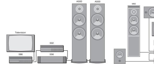
The 586 DVD Player provides a two-channel analogue audio output, normally encoded in Dolby Surround, to allow direct connection to an analogue pre-amplifier such as the 502 Analogue Controller.
