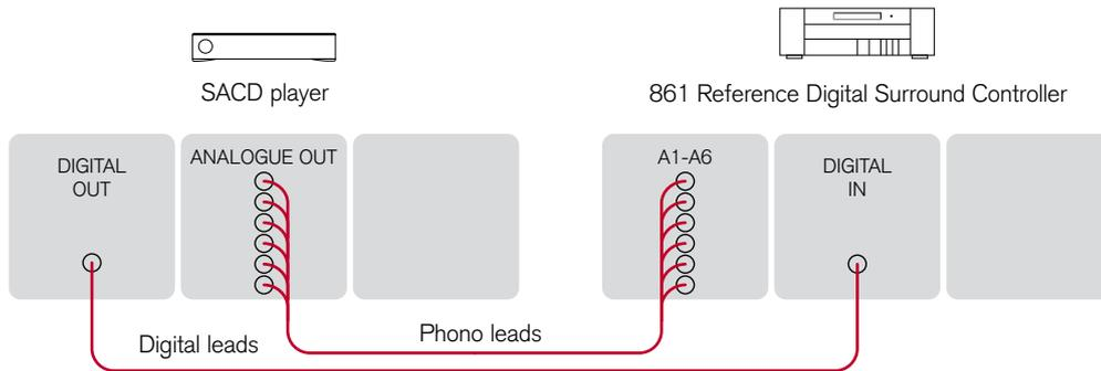
The 861 Reference Digital Surround Controller provides two sets of 6 analogue inputs, called A1-A6 and B1-B6. Each set can be used as a multichannel input from a source with a suitable analogue multichannel output, such as an SACD player.
