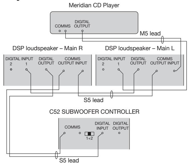
You can connect a pair of DSP loudspeakers and a subwoofer directly to a digital source. The DSP loudspeakers include volume, balance, and tone controls allowing you to control the system using the MSR+.
