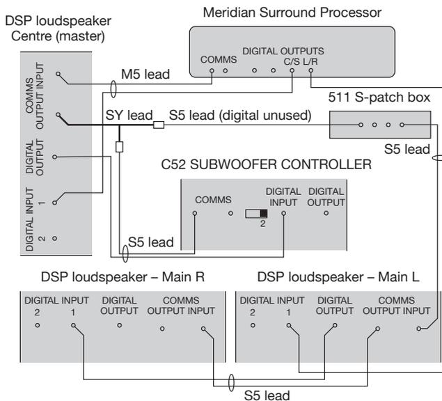
If your system includes more than two Meridian DSP loudspeakers you will need a 511 slave patch box (available separately) to link together the S5 leads from each speaker, as shown above.
