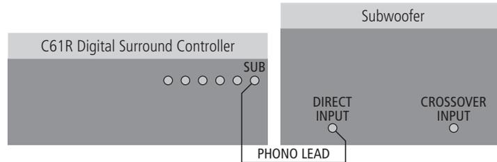
The Meridian SW1600 and SW5500 subwoofers provide both digital and analogue inputs, allowing you to connect them to either the digital or analogue subwoofer outputs of the C61R. The analogue connection must be used if you do not have a digital main speaker.
