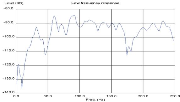
Shows the loudspeaker-room response to a low frequency sine wave, swept between 0 and 250Hz. The ideal low frequency response would be smooth. A peak in the response indicates a resonance at the corresponding frequency. A dip in the response indicates absorption or cancellation at the corresponding frequency.
