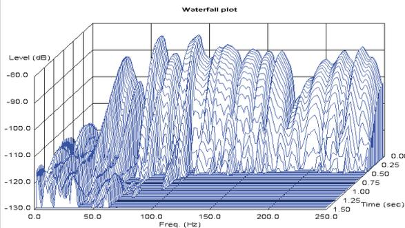
Shows the response of the room to a series of short sine wave pulses of frequencies between 0 and 250Hz. It shows how the response decays over time at each of those frequencies.
