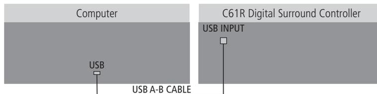
You can connect a Windows PC or Macintosh to the C61R via the USB input to allow you to use the C61R as a digital audio output device.
