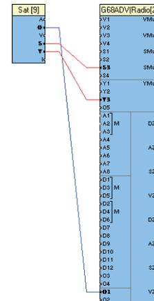
This shows the audio connection between the satellite receiver optical output and the optical input O1 on the digital surround controller, and the S-video and component video connections between the satellite receiver and the digital surround controller.
