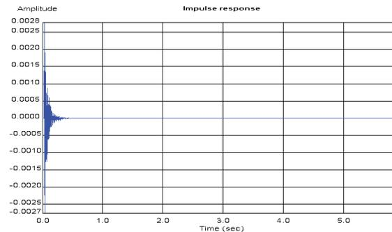
Shows the response over time of the loudspeaker to a click. The curve shows a maximum just after time zero, and then decays rapidly depending on the amount of reverberation in the room. Any additional peaks in the response indicate resonances set up by the initial impulse.
