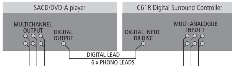
Analogue inputs A1 to A3 can be used as a multichannel input from a source with a suitable analogue multichannel output, such as an SACD player. Analogue inputs A4 to A6 can optionally be used as a second multichannel analogue input.
