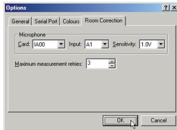
The default number of retries is 3. If the measurements are consistently giving poor SNR figures you can reduce the number of retries. However, it is better to follow the steps described below to improve the measurement conditions. The better the measurement the more accurate the results when calculating the filters for a profile.
