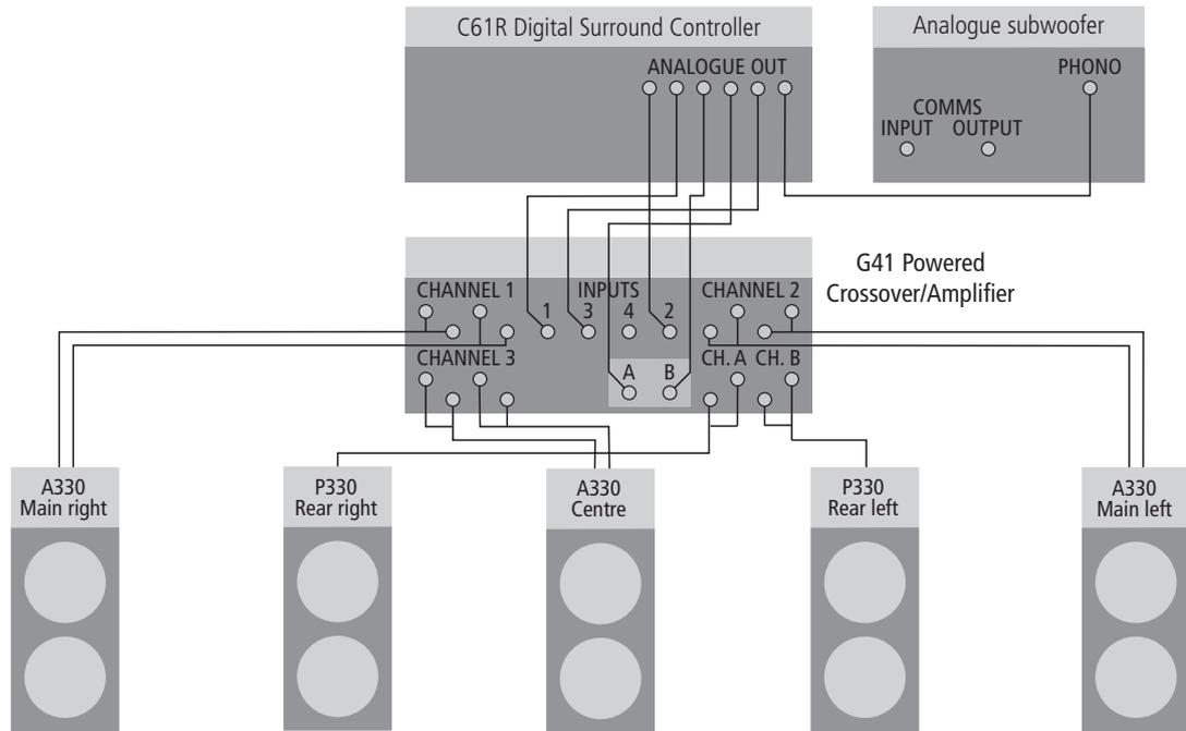
The C61R provides six analogue outputs to allow you to connect to six power amplifiers and passive loudspeakers, or 300 Series Active and Passive Installation Loudspeakers powered by the G41 Active Crossover Amplifier.
