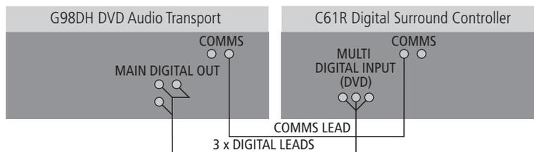
The C61R Digital Surround Controller provides 12 digital coax inputs, six of which can be used as two multichannel inputs from a source with a suitable digital multichannel output, such as the G98DH DVD Player.
