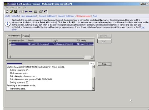
When the measurements have been completed the following dialogue box allows you to apply the room correction profiles:
