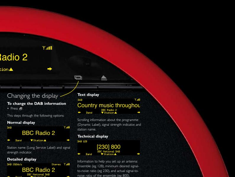
Bit rate (higher is better quality), Stereo/ Mono, signal strength indicator, station name,
