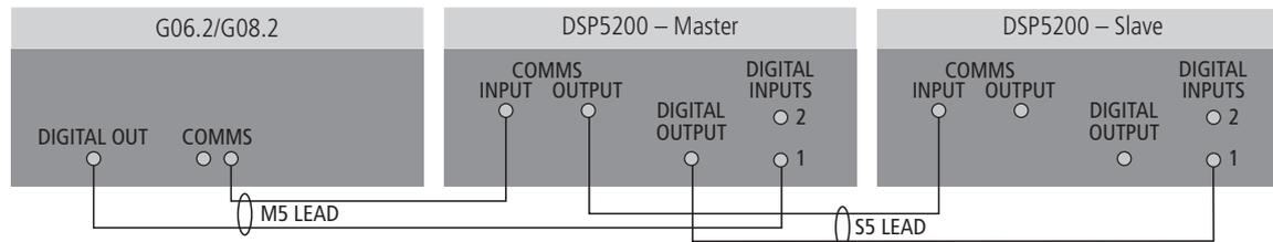
The G06.2 and G08.2 can be connected directly to Meridian DSP loudspeakers to create a complete compact stereo system, with volume and other preamplifier controls provided by the loudspeakers via the MSR+.
