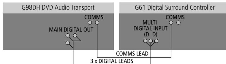
The G61 Digital Surround Controller provides 12 digital coax inputs, six of which can be used as two multichannel inputs from a source with a suitable digital multichannel output, such as the G98DH DVD Player.
