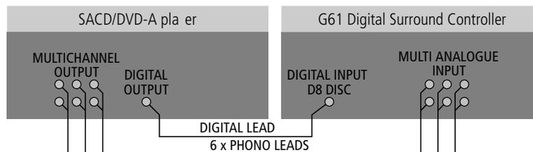
The G61 Digital Surround Controller provides eight analogue inputs, three of which can be used as a multichannel input from a source with a suitable analogue multichannel output, such as an SACD player.
