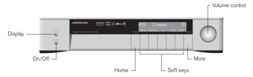
The five soft keys under the display make the G Series products particularly easy to use. They change to reflect what the product is doing. For example, if you are customizing the DSP settings they provide controls to label and store the preset. The current function of each key is shown above the key on the bottom line of the display.
