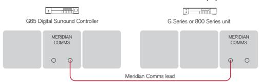
In a system of Meridian products the products should be linked together in a chain, via the COMMS sockets, using the Comms leads supplied with each product. The sequence in which you connect the units is not important.
