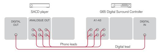
Analogue inputs A1 to A3 can be used as a multichannel input from a source with a suitable analogue multichannel output, such as an SACD player. Analogue inputs A4 to A6 can optionally be used as a second multichannel analogue input.
