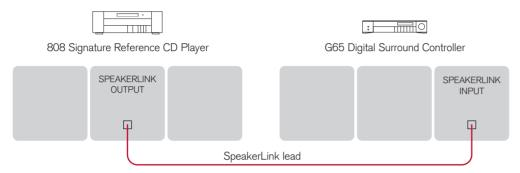
Connect the DIGITAL output from the 808 to one of the SpeakerLink inputs on the digital surround controller, using a Meridian SpeakerLink lead.
