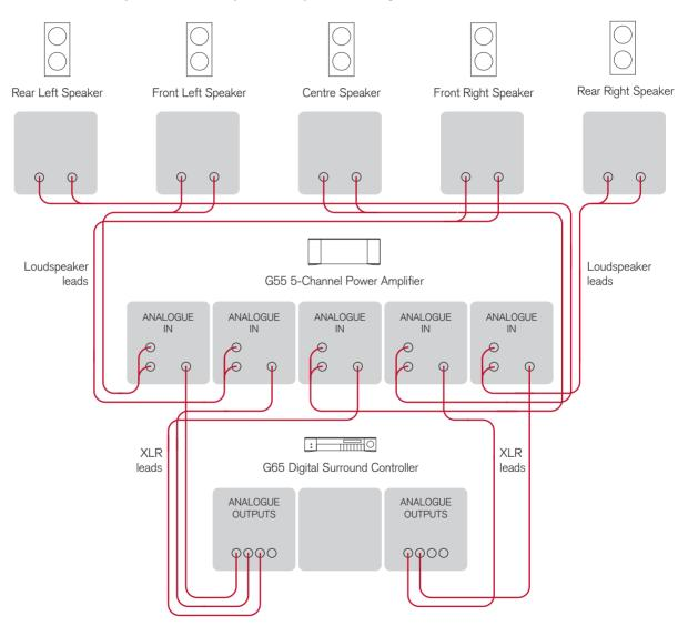
The G65 provides eight balanced analogue outputs to allow you to connect to active loudspeakers, or power amplifiers and passive loudspeakers. An ideal choice is the Meridian G55 5-Channel Power Amplifier.
