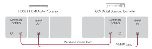
The G65 provides an MMHR multichannel input which can be used with the HD621 HDMI Audio Processor.
