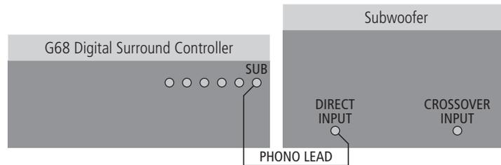
The Meridian SW1600 and SW5500 subwoofers provide both digital and analogue inputs, allowing you to connect them to either the digital or analogue subwoofer outputs of the G68. The analogue connection must be used if you do not have a digital main speaker.
