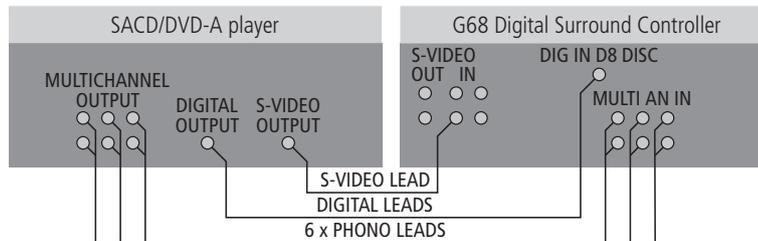
The G68 Digital Surround Controller provides eight analogue inputs, three of which can be used as a multichannel input from a source with a suitable analogue multichannel output, such as an SACD player.
