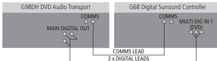
The G68 Digital Surround Controller provides 12 digital coax inputs, six of which can be used as two multichannel inputs from a source with a suitable digital multichannel output, such as the G98DH DVD Player.
