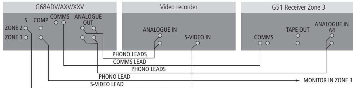
The G68 can copy the currently selected audio and video inputs to two different outputs, called COPY ZONE 2 and ZONE 3, for recording, or for controlling one or two other rooms. For example, a G51 Receiver could be used in a second room to listen to a source connected to the G68.
