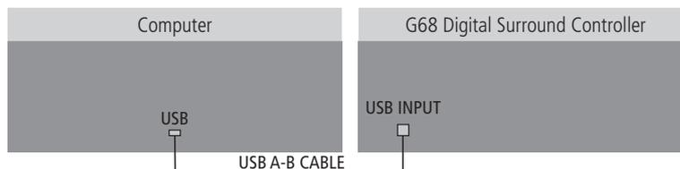
You can connect a Windows PC or Macintosh to the G68 via the USB input to allow you to use the G68 as a digital audio output device.
