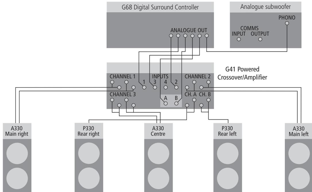
All versions of the G68 provide six balanced or unbalanced analogue outputs to allow you to connect to six power amplifiers and passive loudspeakers, or 300 Series Active and Passive Installation Loudspeakers powered by the G41 Active Crossover Amplifier.
