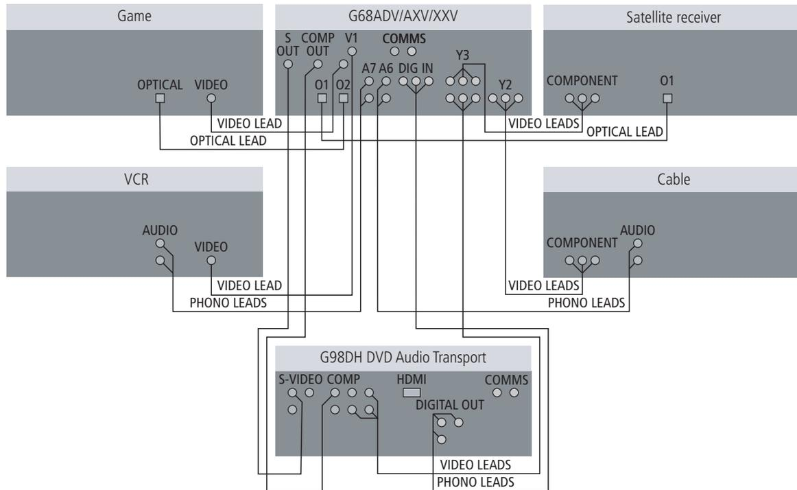
If you are using the G68ADV, AXV, or XXV Digital Surround Controller in conjunction with a G98DH DVD Audio Transport, you can perform video switching in the G68 but take advantage of the video format conversion and scaling in the G98 to drive the display device.
