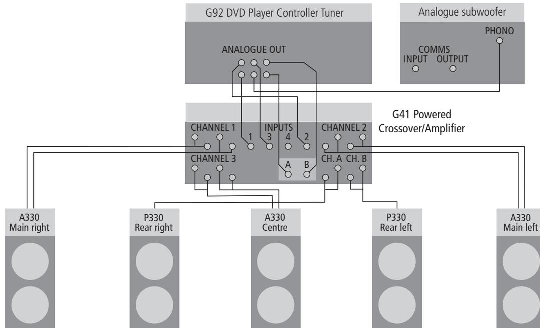
The G92 provides six analogue outputs, and includes surround decoding to allow you to create a 5.1 surround system directly connected to six power amplifiers and passive loudspeakers, or 300 Series Active and Passive Installation Loudspeakers powered by the G41 Active Crossover Amplifier.
