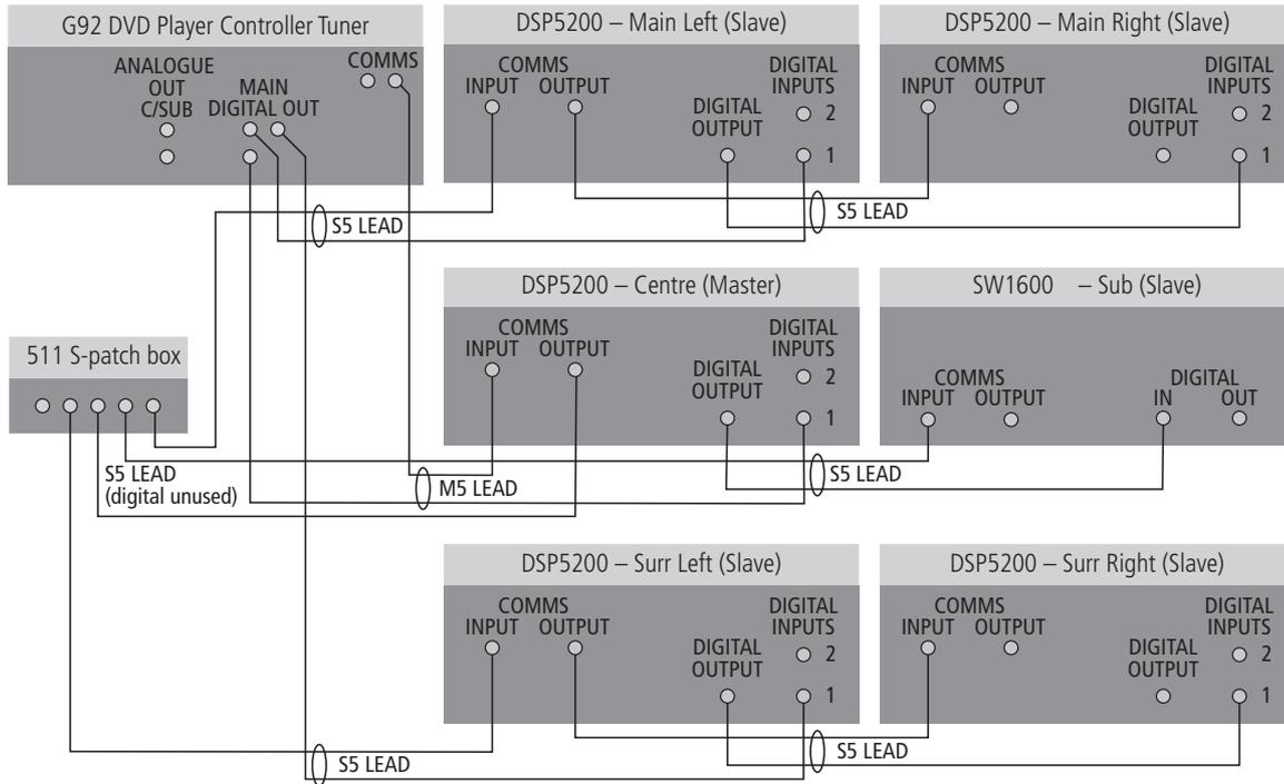
The G92 includes all the digital surround decoding needed to create a 5.1 surround system, directly connected to up to five DSP loudspeakers, such as Meridian DSP5200s, and a DSP subwoofer, such as the Meridian SW1600.
