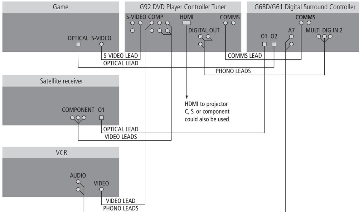
The G Series DVD player can be used in combination with a G68 Digital Surround Controller to create a superb audio/video system, using the video switching and format conversion provided by the DVD player to handle the video, and the audio switching provided by the G68D/G61 to handle the analogue and digital audio.
