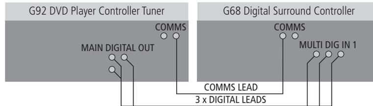
The multichannel digital output is the preferred way of connecting to a 96kHz and MHR capable Meridian digital surround processor, such as a 568.2, G68, or 861, as it provides additional MHR SMART LINK information about the source format.
