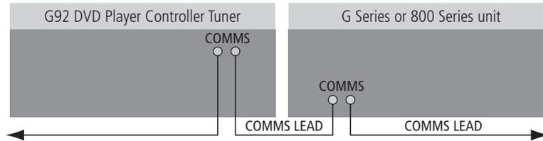
In a system of Meridian products the products should be linked together in a chain, via the COMMS sockets, using the Comms leads supplied with each product. The sequence in which you connect the units is not important.
