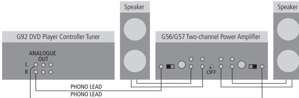
The G92 includes an integrated preamplifier, allowing you to connect it directly to a pair of analogue active loudspeakers, or to analogue passive loudspeakers via a power amplifier such as the G56 or G57.
