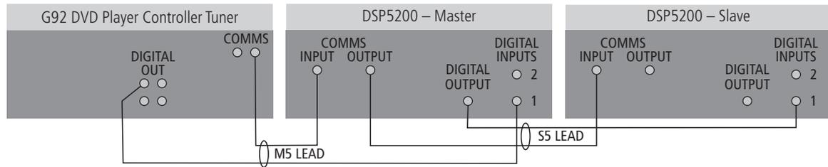
The G92 DVD Player Controller Tuner can be connected directly to Meridian DSP loudspeakers to create a complete compact stereo system, with volume and other preamplifier controls provided by the loudspeakers via the MSR+ or the front panel. The G92 provides additional analogue and digital inputs allowing you to use it to control the other sources in your system.
