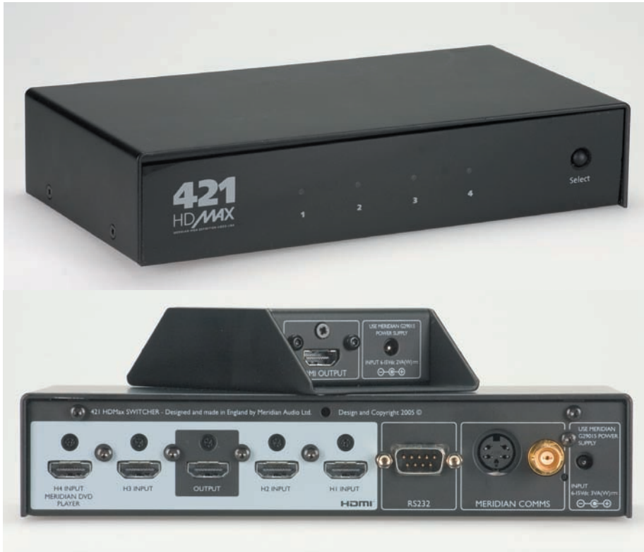
HD MAX 421 Switch (top) and 121 Extender (right). Above: rear panels showing connections. Not to the same scale.
