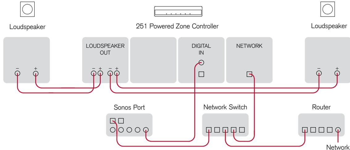
This is a simple, standalone system replaying audio from a Sonos or Roon streaming system.
