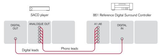
The 861 Reference Digital Surround Controller provides two sets of 6 analogue inputs, called A1-A6 and B1-B6. Each set can be used as a multichannel input from a source with a suitable analogue multichannel output, such as an SACD player.
