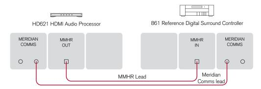
The 861 provides an MMHR multichannel input which can be used with the HD621 HDMI Audio Processor.
