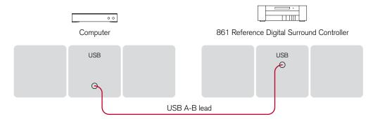
You can connect the 861 Reference Digital Surround Controller to a PC or Macintosh USB socket to allow you to use the 861 as a digital audio output device.
