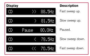
The sine sweep will stop when it reaches 0.5Hz or 200Hz.
