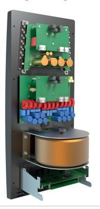
The amplifiers for the tweeter and mid-range driver are Class-AB designs capable of delivering 150W into  $4\Omega$  with extremely low noise and distortion under all conditions.
