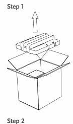
Ensure the carton is standing on its base; this can be confirmed by checking that the information printed on the carton is the right-way up.
