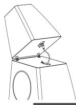
Next, lift the rear of the head-unit slightly to allow the short connecting cable to be located and plugged into the socket on the underside of the head-unit. This connection is latched, so a click should be felt as the cable is pushed fully home.
