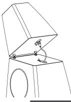
Next, lift the rear of the head-unit slightly to allow the short connecting cable to be located and plugged into the socket on the underside of the head-unit. This connection is latched, so a click should be felt as the cable is pushed fully home.
