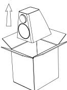
Taking care not to apply pressure to the drive units, the head-unit can now be lifted out of the carton and placed carefully on an appropriate surface.
