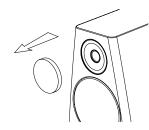
When the loudspeaker is ready to be used, remove the tweeter-cover and retain it so it can be used if required at a later date.
