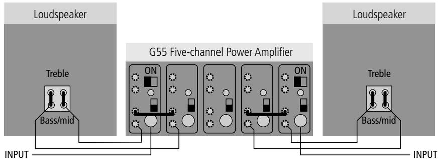
You can wire channels 1/2 and 4/5 in bridge output mode, to obtain more than twice the power output.
