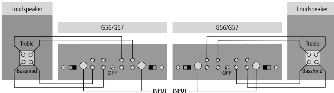
Extremely high sound quality can be achieved using two separate G56/G57 Two-channel Power Amplifiers, one to drive each loudspeaker. The two channels in each G56/G57 Two-channel Power Amplifier are used to drive the LF and HF units in each loudspeaker.
