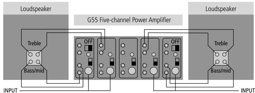
Extremely high sound quality can be achieved using two separate channels of the power amplifier to drive the LF and HF units in each loudspeaker.
