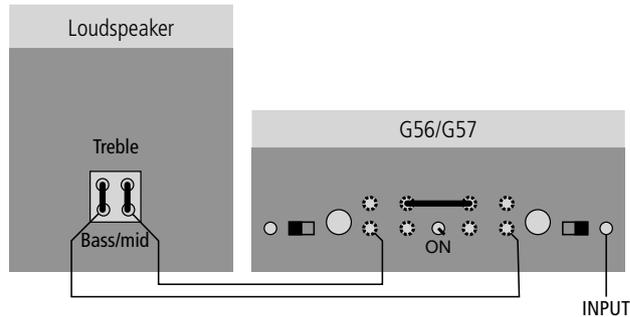
You can use the G56/G57 as a mono power amplifier, to obtain more than twice the power output, by wiring it in bridge mode.
