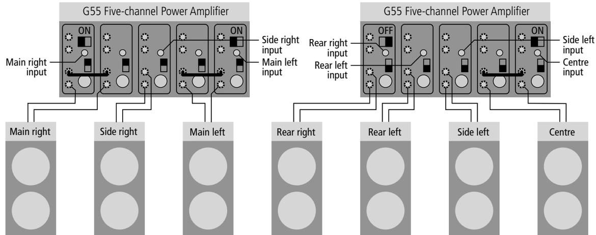
Two G55 Five-channel Power Amplifiers can be used as the basis of a superb seven-channel surround system, taking advantage of bridge mode operation to give more than twice the power output for the three front channels.
