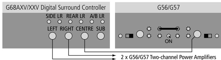
Three G56 or G57 Two-channel Power Amplifiers can be used in bridge mode for each of the front channels of a G68AXV or G68XXV Digital Surround Controller, which are provided as balanced outputs.
